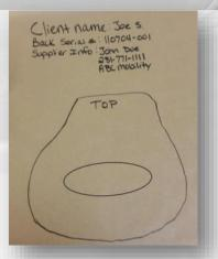
4. Mark which end is the top and draw an approximation of the location and size of the opening cover. Screw holes will need to be added in the field upon installation.
